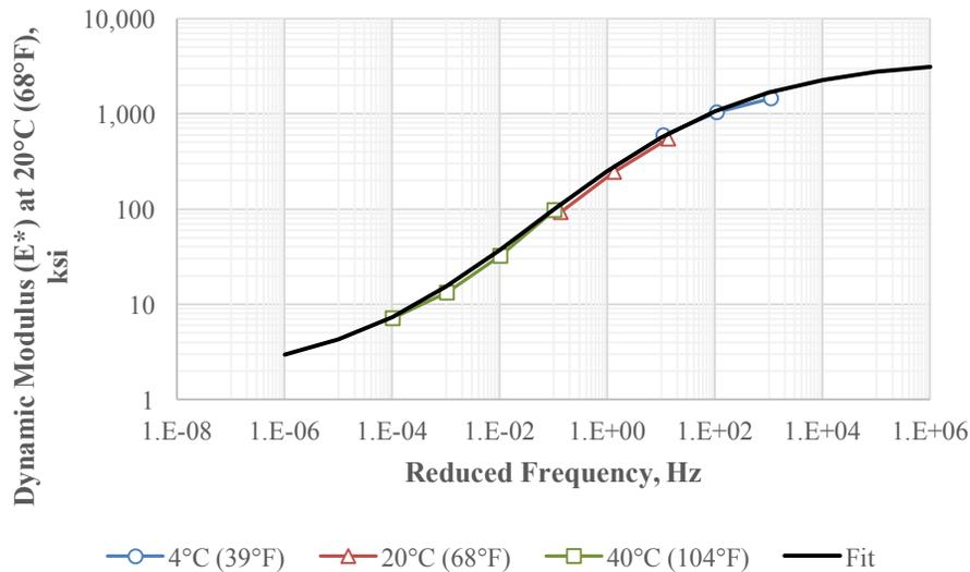
Figure 6. Typical dynamic modulus master curve for HMA mixture.
