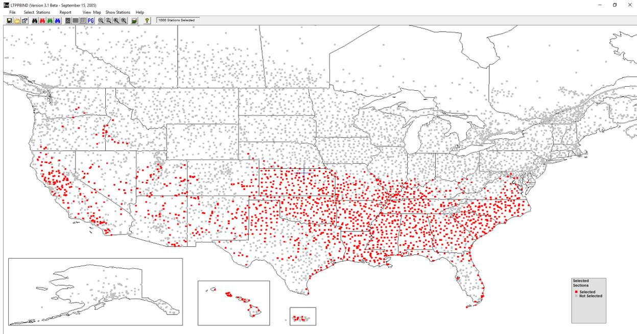
Figure 10. US map from LTP Bind Version 3.1 software showing in red the sections with a high adjusted PG temperature of 64°C.
