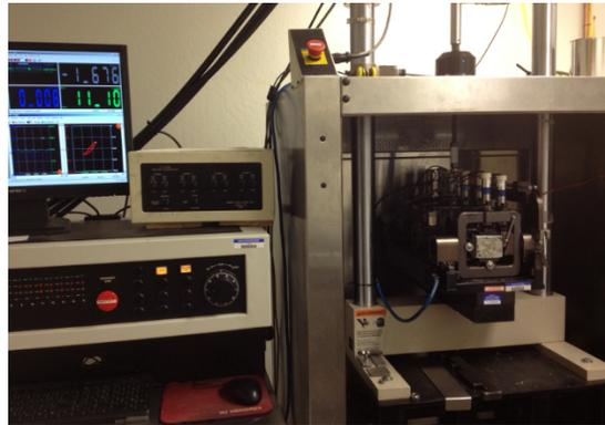
Figure 20. Flexural beam fatigue test setup.
