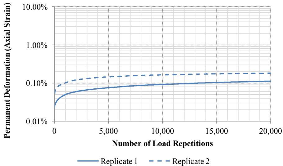
Figure 11. FN test results for the G5-stabilized aggregate mixture.
