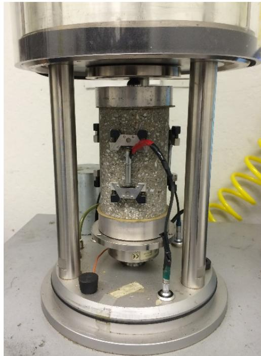
Figure 2. The G5-stabilized aggregate sample in the dynamic modulus testing set-up.
