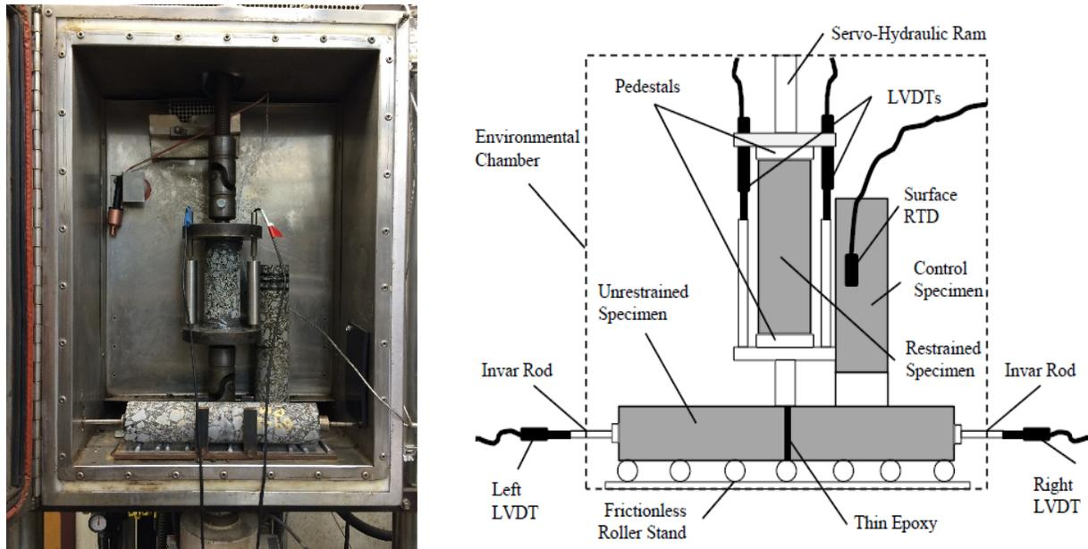
Figure 15. Uniaxial thermal stress and strain test (UTSST) set-up for HMA.
