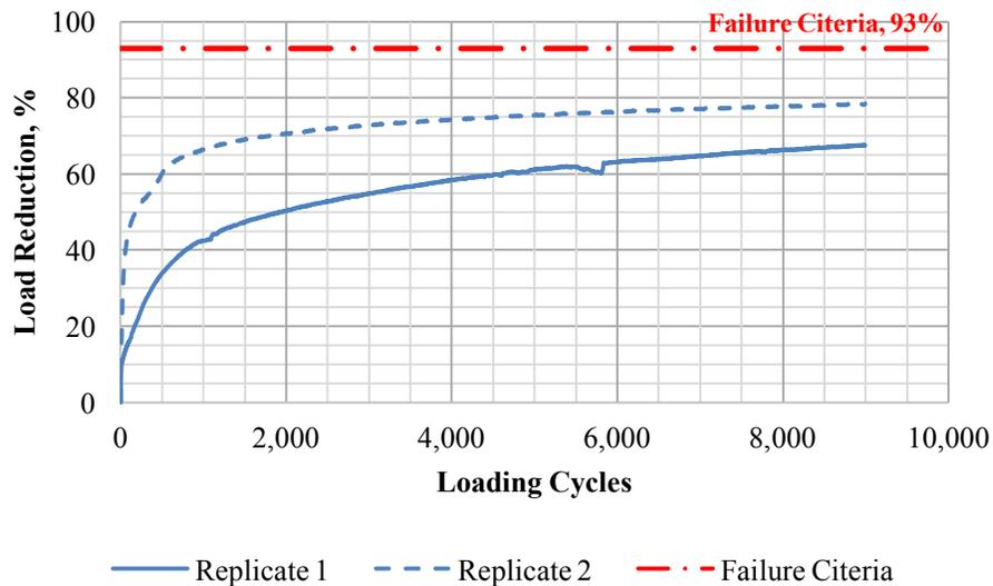
Figure 14. Reflective cracking test results at 10°C (50°F) for the G5-stabilized aggregate mixture.
