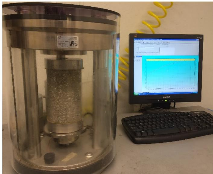
Figure 7. The G5-stabilized aggregate sample in the FN testing set-up
