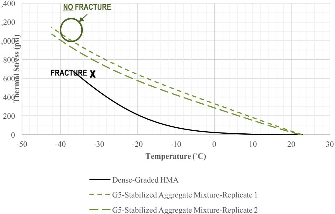
Figure 17. UTSSST thermal stress build-up as a function of temperature for the G5-stabilized aggregate mixture and a typical dense-graded HMA.
