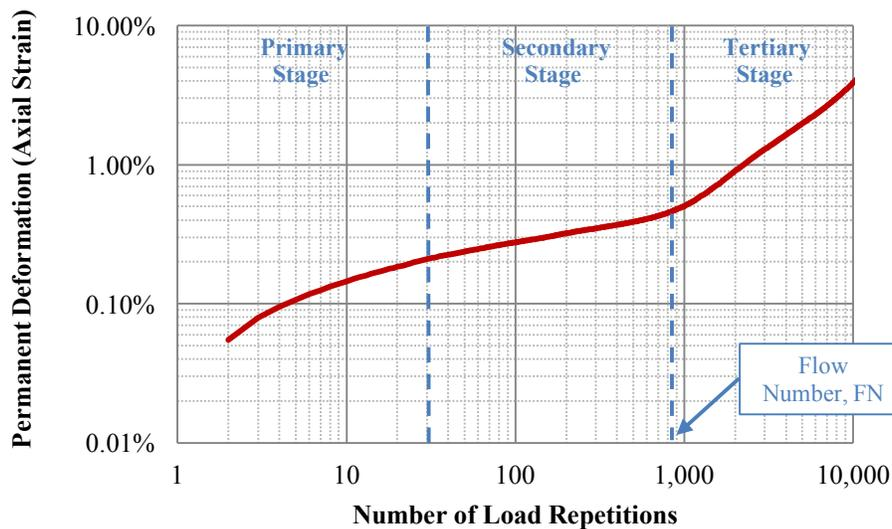
Figure 8. Typical permanent deformation curve for a dense-graded HMA mixture.
