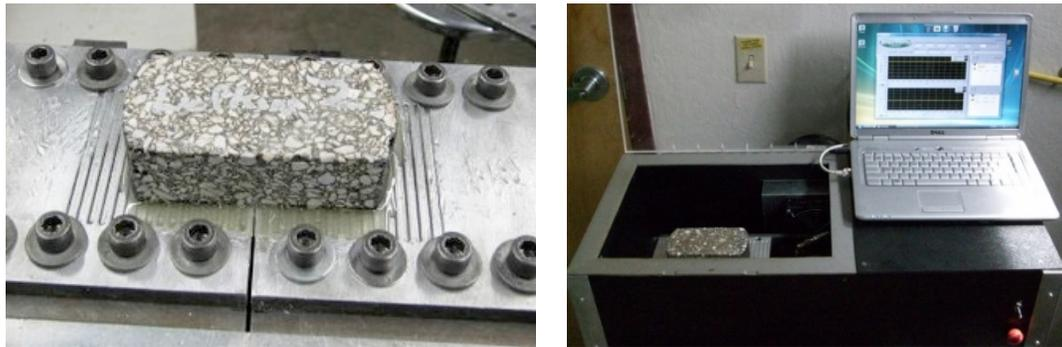
Figure 12. Schematic and photo of the TTI overlay tester.
