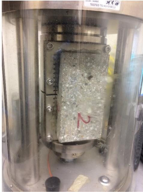
Figure 13. The G5-stabilized aggregate sample in the AMPT overlay testing set-up
