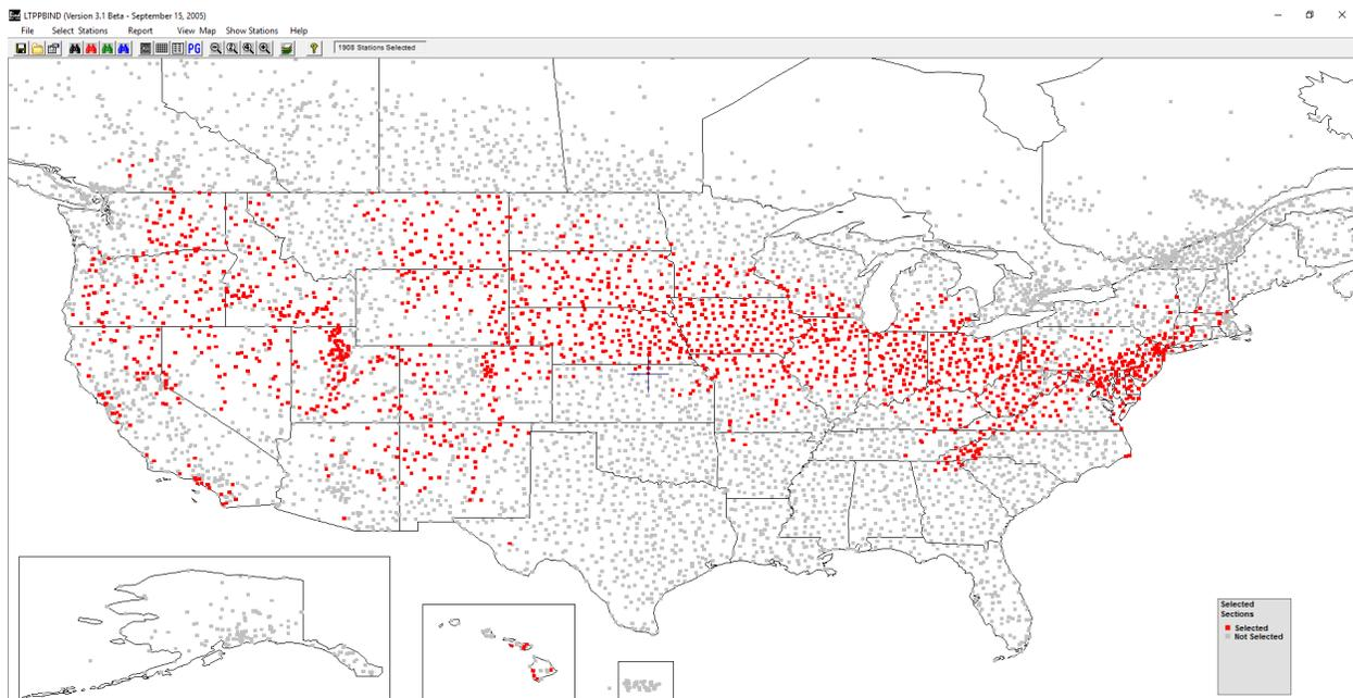
Figure 9. US map from LTPP Bind Version 3.1 software showing in red the sections with a high adjusted PG temperature of 58°C.
