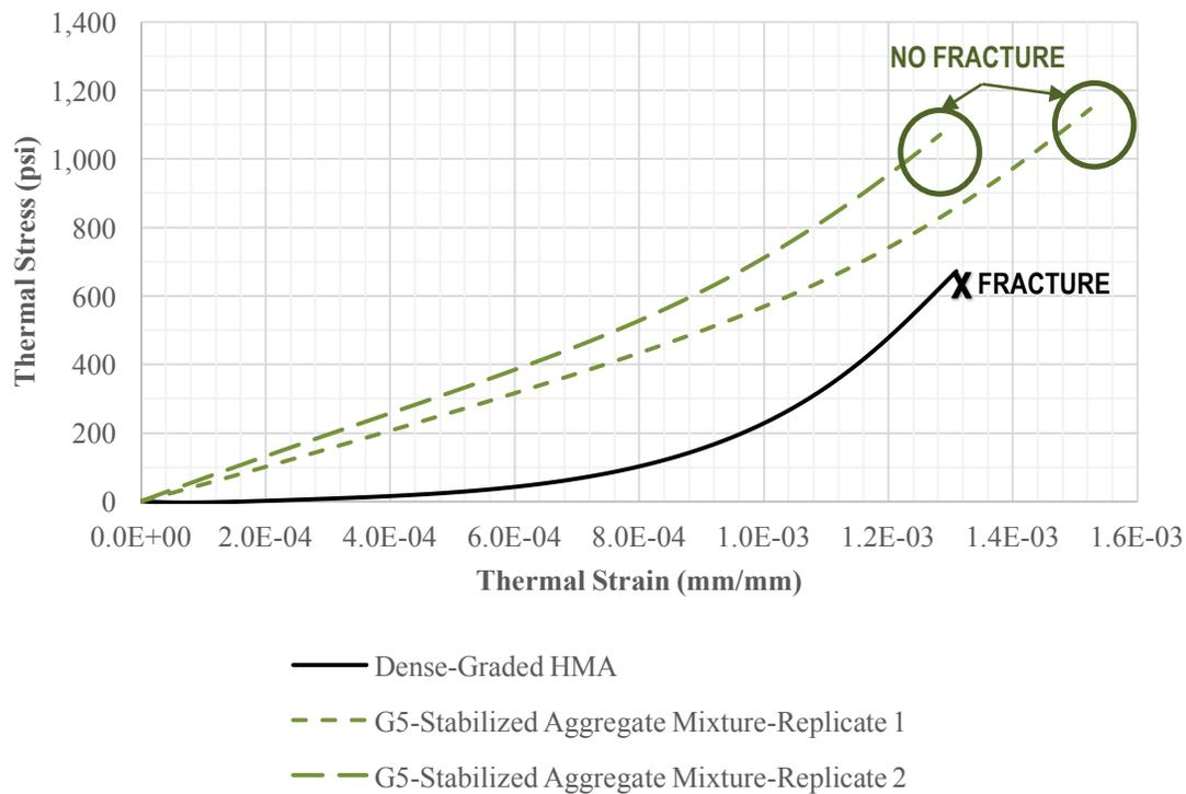
Figure 18. UTSST thermal stress versus thermal strain for the G5-stabilized aggregate mixture and a typical dense-graded HMA.
