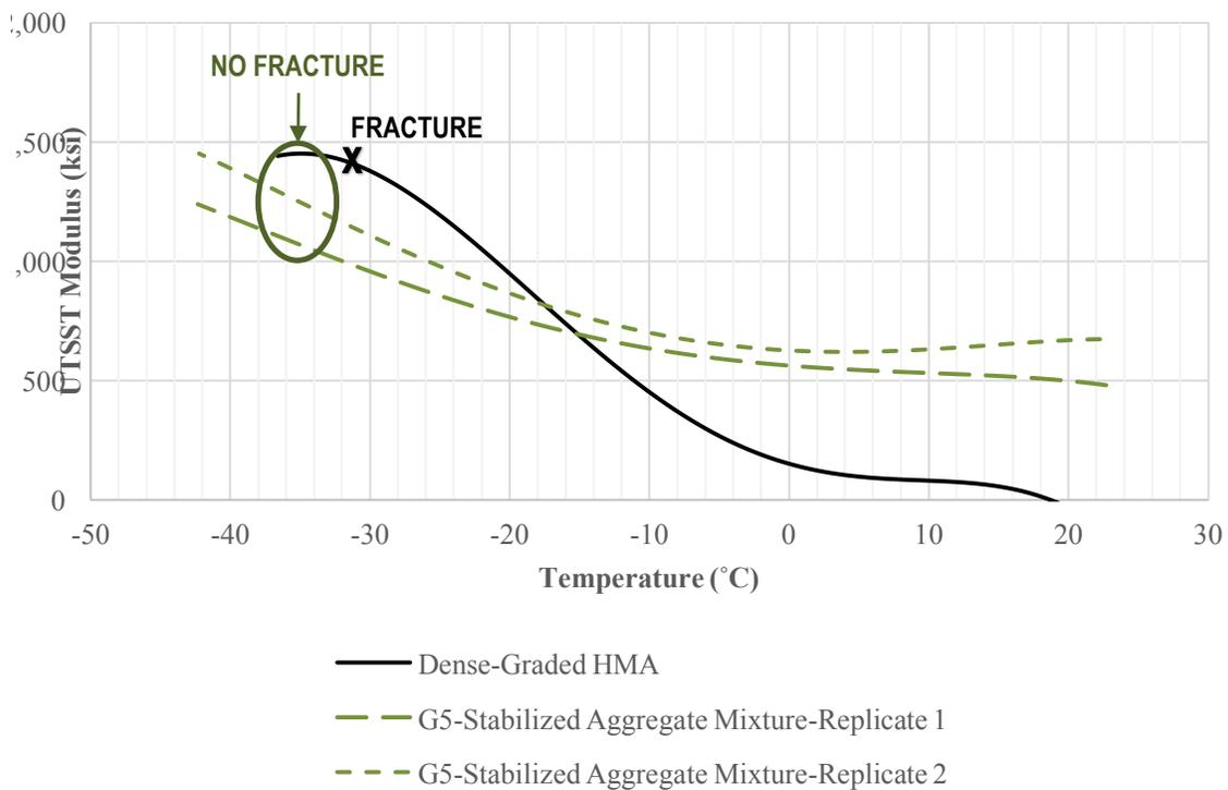
Figure 19. UTSST Modulus for the G5-stabilized aggregate mixture and a typical dense-graded HMA.
