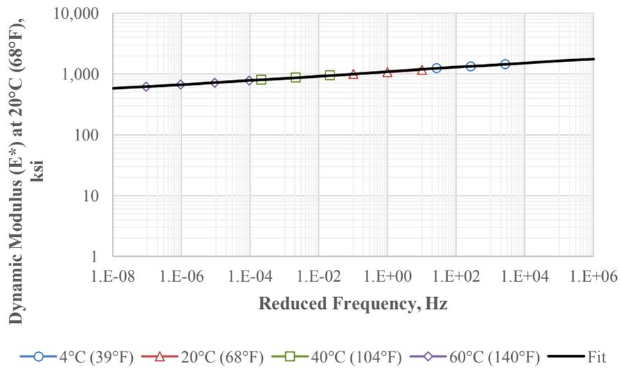
Figure 5. Dynamic modulus master curve for the G5-stabilized aggregate mixture.
