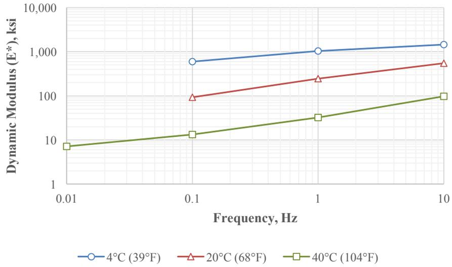
Figure 4. Typical dynamic modulus for HMA mixture.
