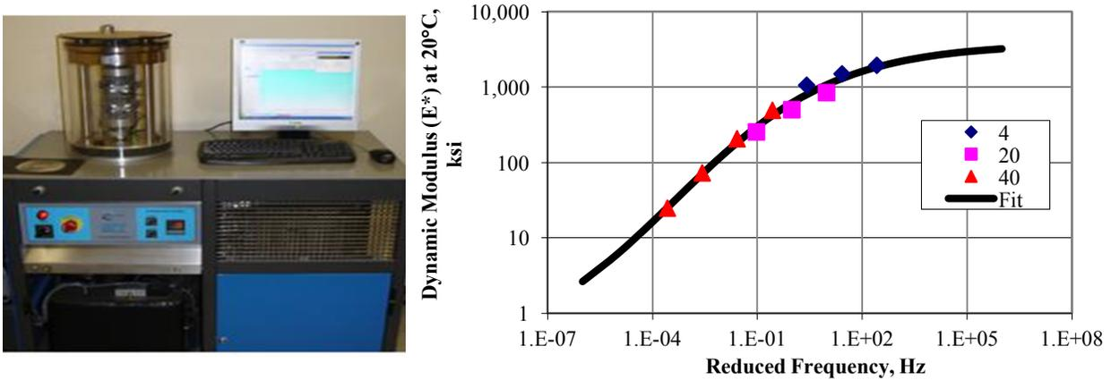
Figure 1. Asphalt mixture performance tester (AMPT) and a typical master curve for asphalt mixture.
