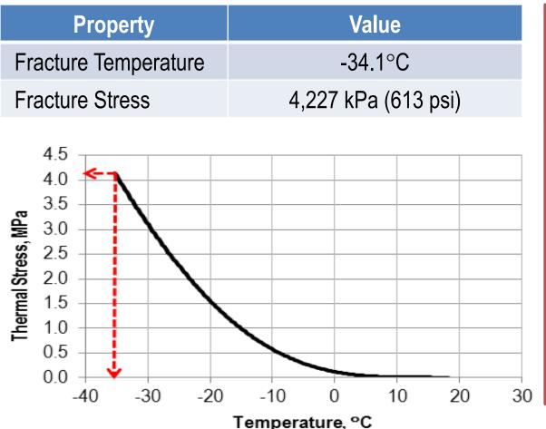
G5<sup>®</sup>-stabilized RAP mixture exhibited a *low* fracture temperature while maintaining a high fracture stress indicating a good resistance to thermal cracking in cold climates.
