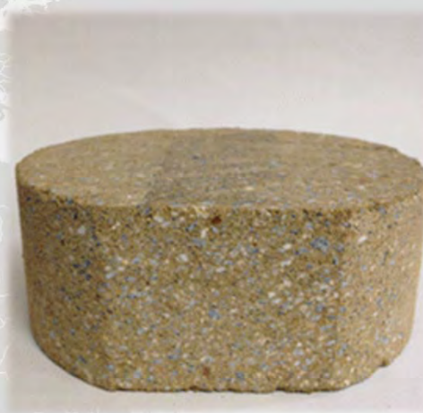
G5 1/4" mixture (25,000 passes, 0.3 mm rut depth)
