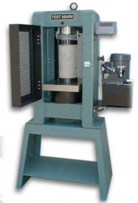
Concrete Compression Test Mark
