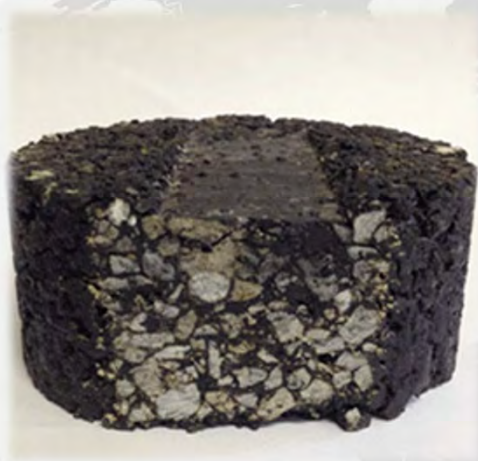
Asphalt Pavement (25,000 passes, 10 mm rut depth)
