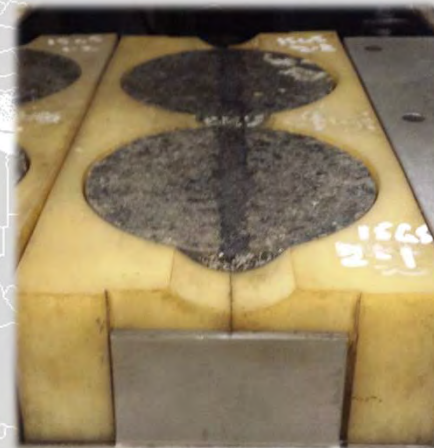
G5 / Recycled Asphalt Pavement (8,000 passes, 0.5 mm rut depth)
